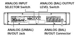
Two kinds of connection as follows are possible by switching the ANALOG INPUT SELECTOR switch.
