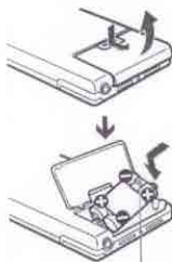
The projection on the battery comes on the right.
