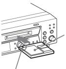
With the label side up, and the shutter on the righthand side.
