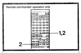
While the MD is playing, press A-B at the start (point A) of the portion to be repeated. Point A is stored.
