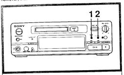
While the unit is in pause mode, hold down FOT for about a second until "All erase?" lights up.
