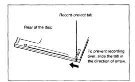
Open the slot to prevent recording. Close the slot to allow recording.
