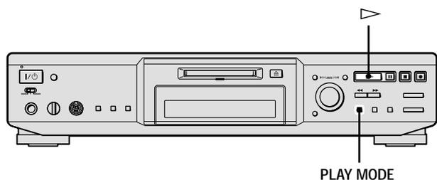
**1** While the deck is stopped, press **PLAY MODE** repeatedly until “SHUF” lights up in the display.
