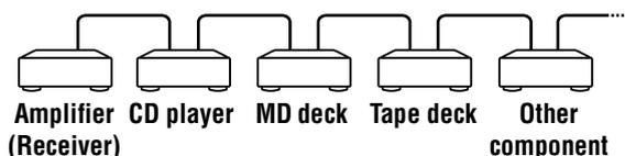
In the CONTROL A1II control system, the control signals flow both ways, so there is no distinction of IN and OUT jacks. If a component has more than one CONTROL A1II jack, you can use either one, or connect different components to each jack.
