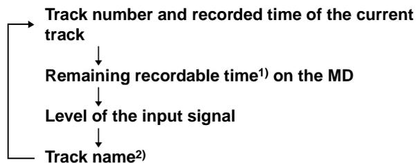
1) Time shown in the display differs depending on the setting of REC MODE.
