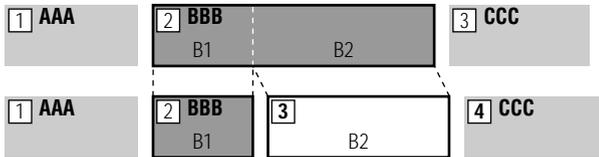
When you divide a track, the total number of tracks increases by one and all tracks following the divided track are automatically renumbered.
