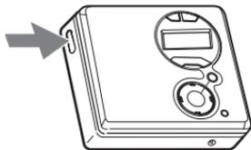
② Insert an MD with the label side facing front, and press the lid down to close.
