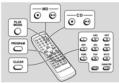
When in the CD or MD mode, press the direct buttons to select the desired tracks.
