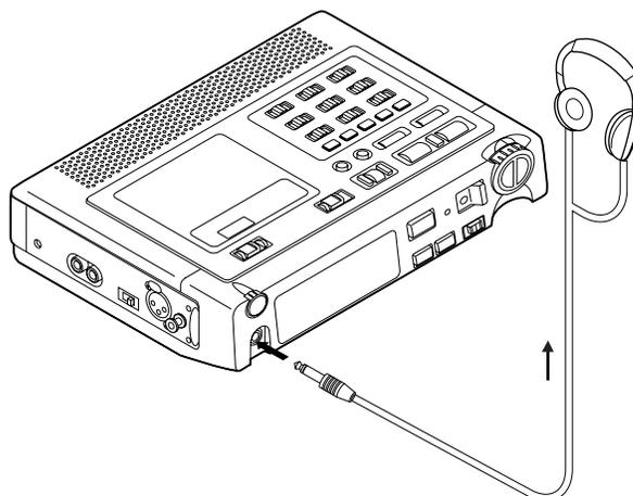
Use the HP/SPK VOLUME knob to control the volume of the headphones. The sound from the internal speaker is muted automatically when headphones are connected.
