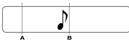
Pressing A-B/DEL during A-B repeat changes point B to point A. (Step ④)
