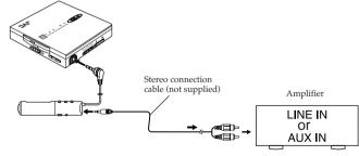
• Direct connection without passing through the remote control may generate noise
