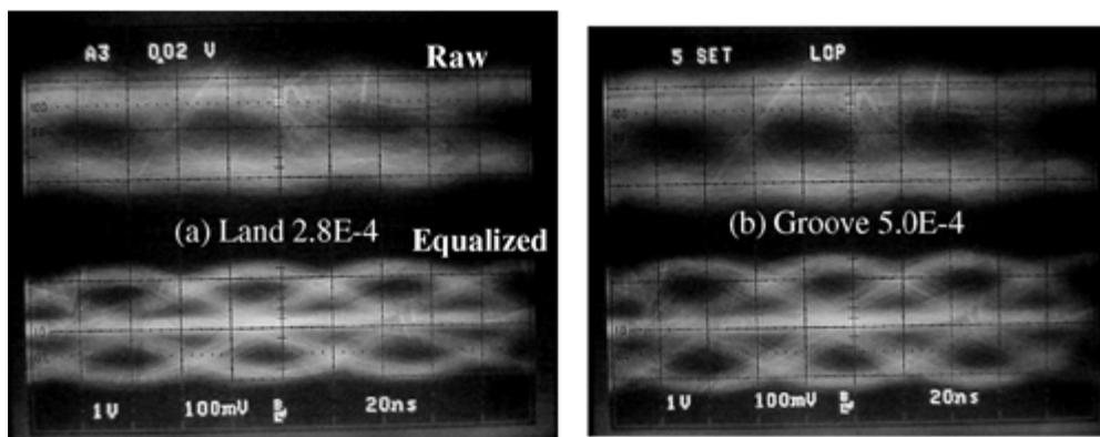
**Fig.3** : Eye pattern at 0.108  $\mu\text{m}/\text{bit}$ .
