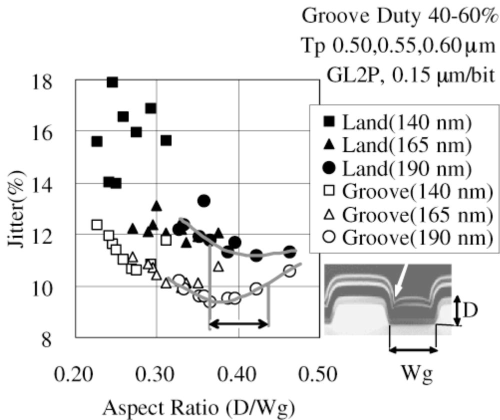
**Fig.5** : Jitter dependence on groove geometry.
