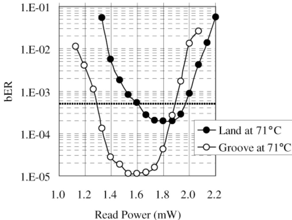
**Fig.10** : Read power margin at  $71^\circ\text{C}$ .
