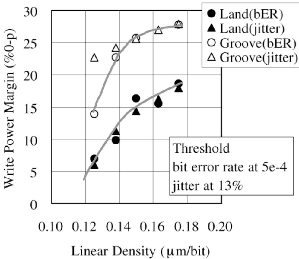
Fig.8 : Power margin on dependence on linear density.
