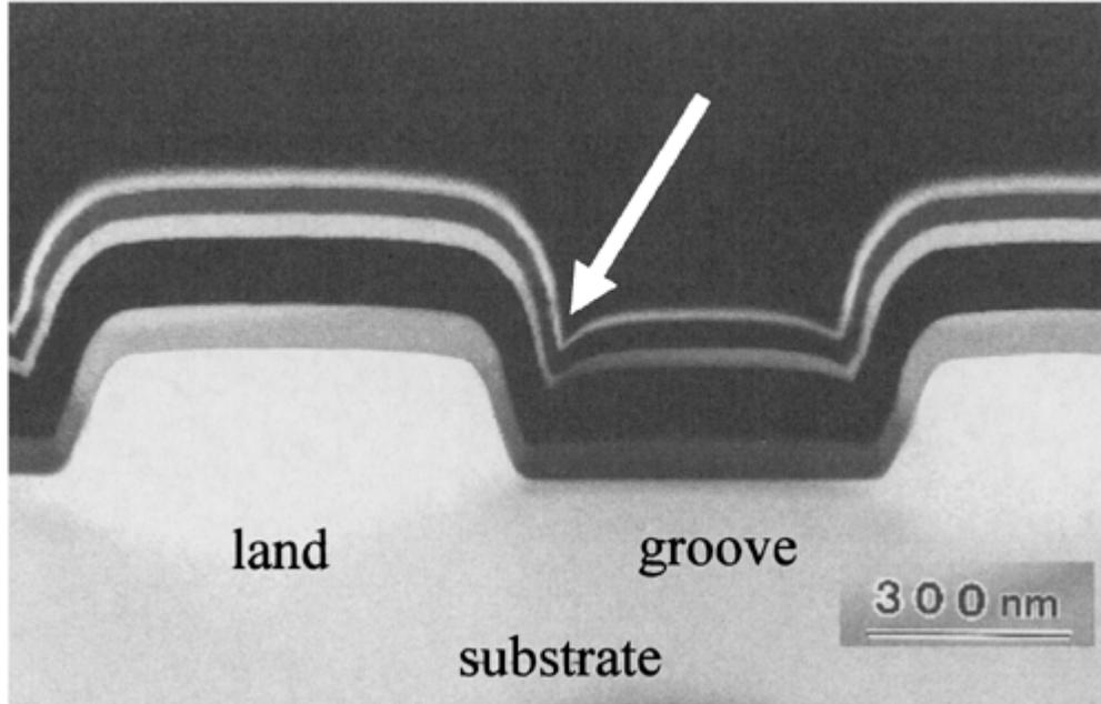
**Fig.1** : Cross section of disk.
