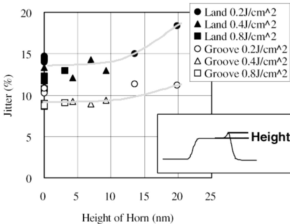
**Fig.7** : Jitter dependence on horn height.
