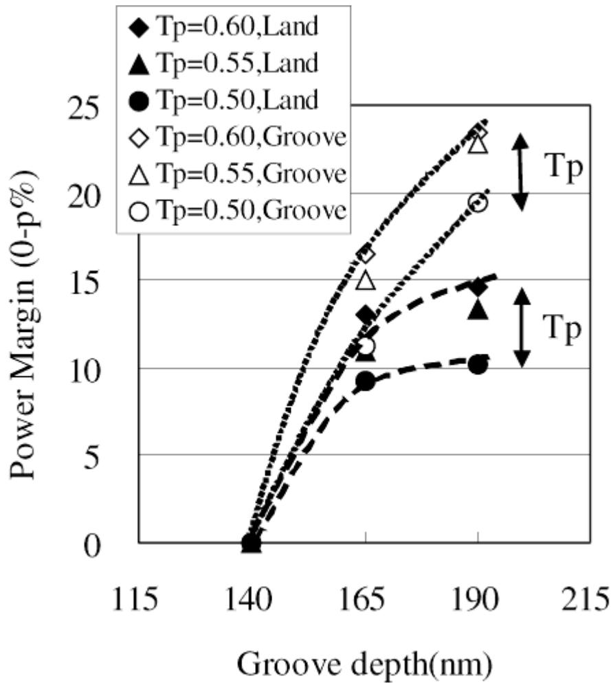
**Fig.6** : Power margin dependence on groove depth and track pitches.
