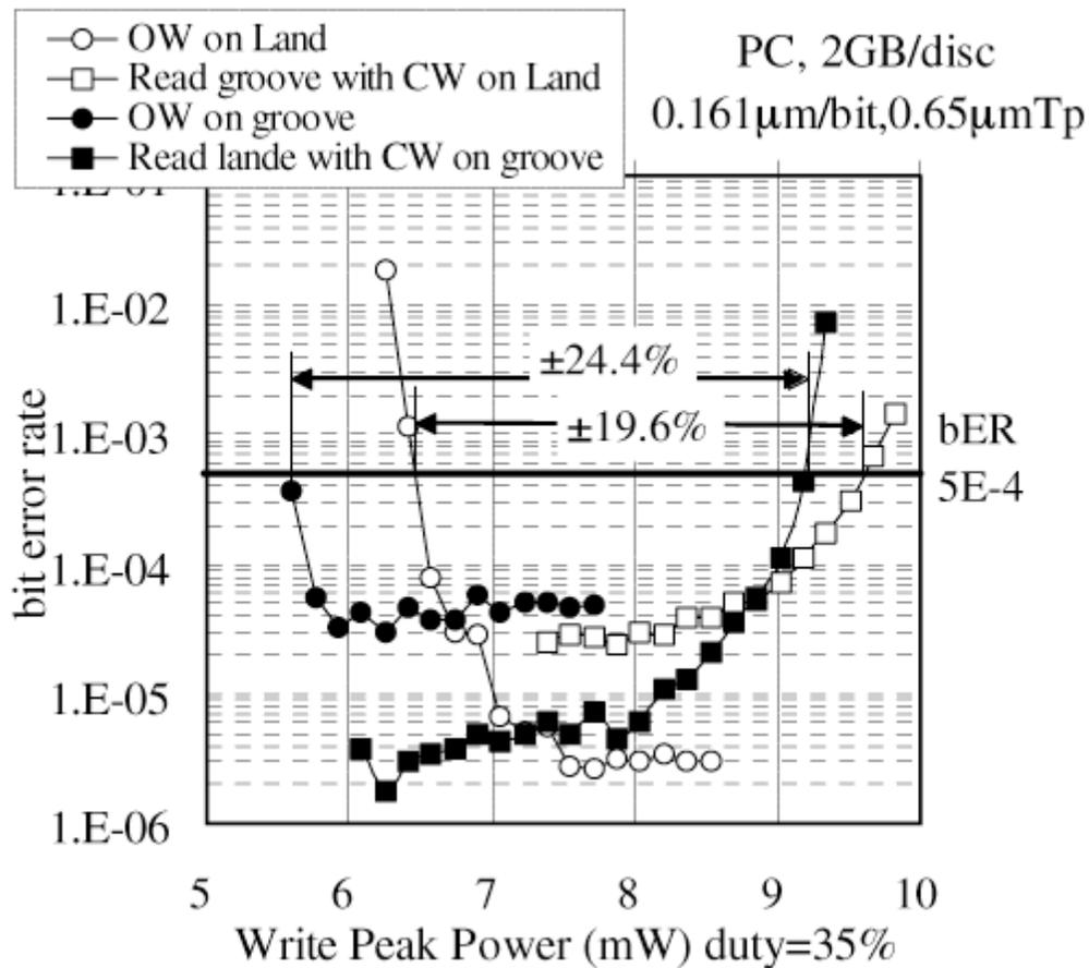
Fig.9 : Write power margin at 2 GB/disc.
