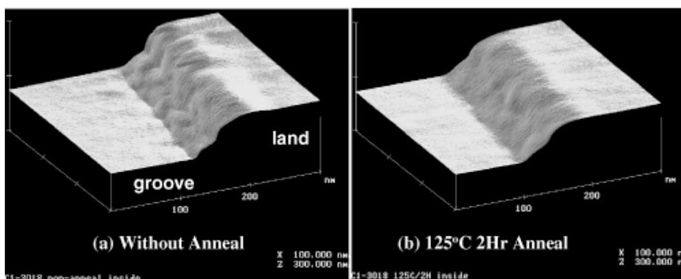
**Fig.4** : AFM images of PC substrate.
