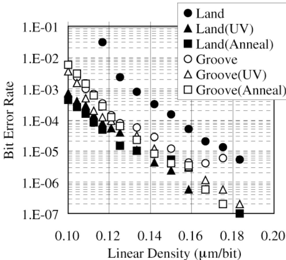
**Fig.2** : Bit Error Rate dependence on linear density.
