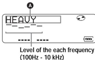
Level of the each frequency (100Hz - 10 kHz)
