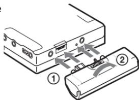
Insert a LR6 (size AA) alkaline dry battery.
