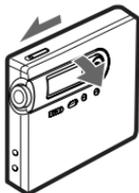
2 Insert an MD with the label side facing front, and press the lid down to close.
