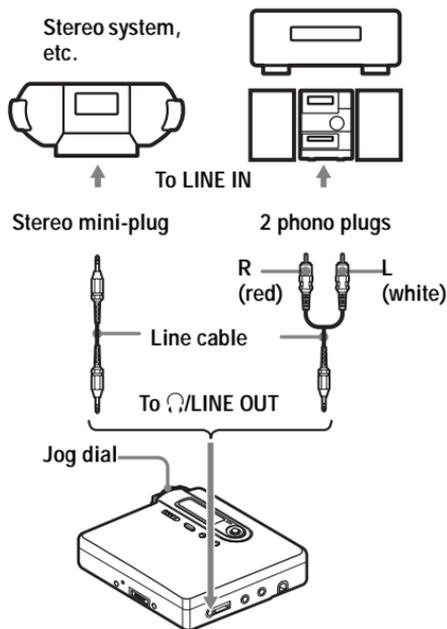
When connecting a line cable to the
