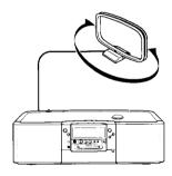
To minimize noise interference from the player section, locate the AM loop antenna away from the player during AM program reception.
