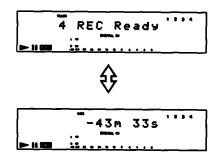
If you changed the recording mode to All REC ON, "AllREC Ready" will alternate with the remaining time on the disc in the display window.
