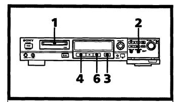
With the label side up and the arrow pointing toward the opening, slide the recordable MD into the disc compartment until the unit grips it.
