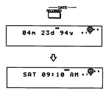
"No Date" appears if the built-in clock has not been set or the track was recorded on another unit without a date and time stamp function. The previous display reappears when you press DATE RECORDED again or after a few seconds have passed.
