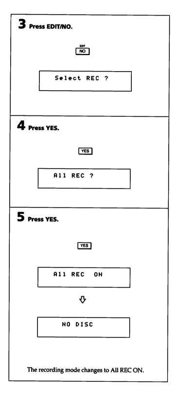
Restoring the recording mode to its factory setting Repeat the above procedure, pressing EDIT/NO in step 5 to change the recording mode to All REC OFF.
