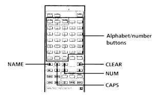
1 Press NAME repeatedly until a flashing cursor appears in the display, then do the following:
