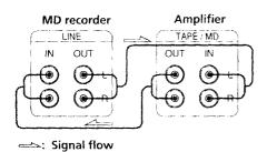
Connecting the recorder to a digital component such as a CD player, DAT deck, digital amplifier, or another MD recorder
