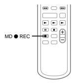
→ Press MD • REC during recording at the point you want to add a track mark. The tracks following the added one are renumbered.
