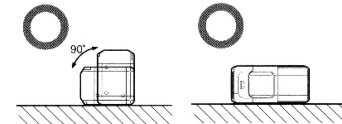
Do not install the unit on a detached mounting board for placement on uneven surfaces or upside down.
