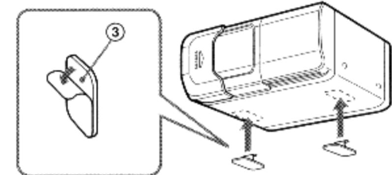
**2** Remove any dirt or stains from the surface you're going to mount the unit on, then attach the unit.
