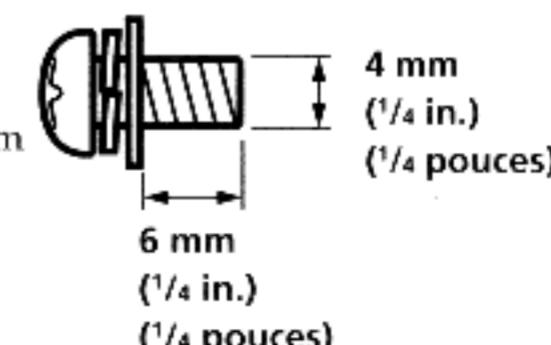
To prevent damage to the unit, do not use screws longer than 6 mm (1/4 in.).
