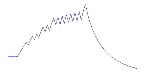
Example: Reading the sample of the "power" button in Sony RM-SMD1 Remote Control As we can see, before the sample the line level is around 0. There is no signal at this point; therefore the first change is when there is signal – and the change is upwards. The line level goes upward for about 2.4 milliseconds, then goes down for 0.6 milliseconds. This means the IR signal was on for 2.4 milliseconds and then off for 0.6 millisecond. The whole signal was:
